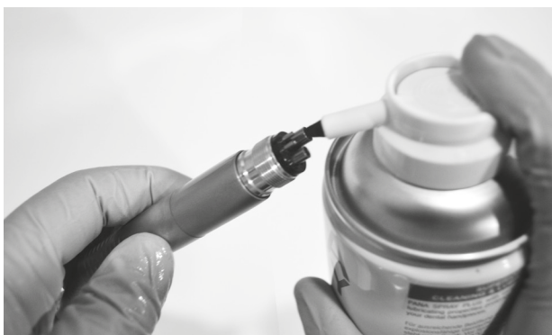
Injecting maintenance oil into the spray channel (maintenance oil item no. 4801326 and spray channel adapter item no. 4801328)
